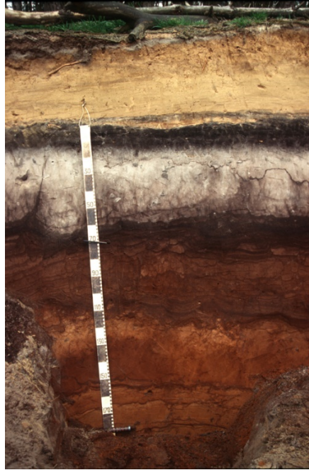
Figure 3. A soil profile showing clear changes in composition and color as depth increases. Many sediments do not show such an obvious change, so samples must be taken with care to fully represent the evidence and avoid mixing of layer samples.
